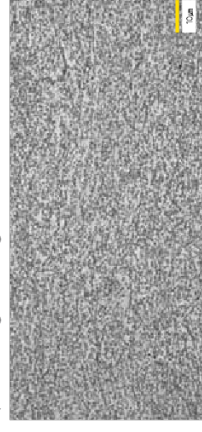
Spherical cementites in ferrite matrix
